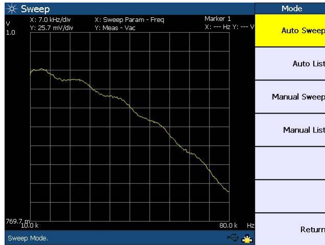
Figure 7-3 Sweep mode selection
